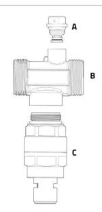
Installation The device must only be installed in a vertical position, with the drain hole facing downwards, to allow the drained water to flow out properly in opening mode.
